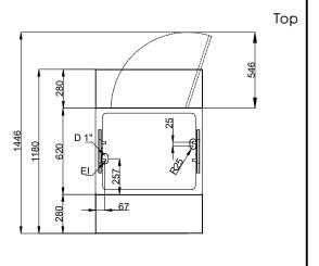
Electric Supply voltage: 220-240 V/1N ph/50/60 Hz Electrical power max: 2.04 kW Water: Water drain outlet size: 3/4" **Key Information:** N° of doors: External dimensions, Width: 770 mm 1180 mm External dimensions, Depth: External dimensions, Height: 1304 mm Net weight: 94.5 kg Shipping height: 1420 mm Shipping width: 910 mm Shipping depth: 830 mm Shipping volume: 1.07 m<sup>3</sup> +85 / +9<u>5</u> °C Set temperature:
